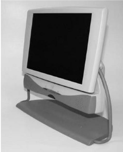
The **DT500** Home Internet Access Device by *DT Research* (DTR) is a LCD-based thin-client platform aimed at providing easy and efficient access with custom user-interface to a variety of applications and services over the Internet. The **DT500** is powered by Linux or Windows CE technology to deliver the responsive experience and stable environment expected of consumer and home appliances.
