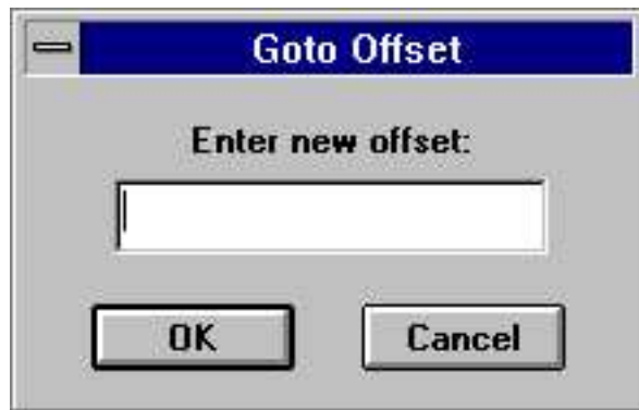
Figure 138. In the Goto Offset dialog, enter the offset you want to appear at the top of the Memory Display window.
