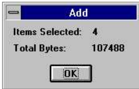
Figure 141. As you select objects, the Add function calculates and displays the number of selected objects and their total size.
