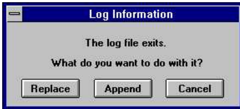
Figure 172. The Log Information message box appears when logging if the Query option is selected on the Log Configuration dialog.
