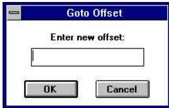
Figure 199. In the Goto Offset dialog, enter the offset you want to appear at the top of the Memory Display window.
