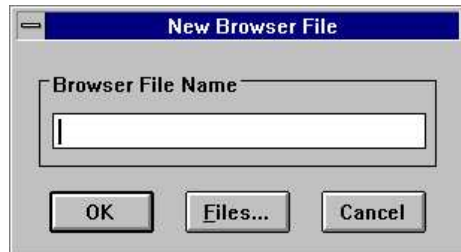
Figure 30. Use the New Browser File dialog to create a new Browser database file.
