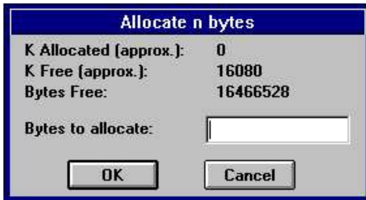
Figure 148. On the allocation dialog box, enter the desired amount of memory to allocate, free, or leave unallocated.
