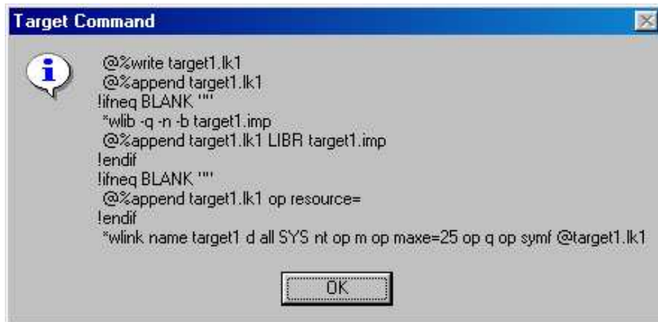
Figure 19. The Target Command dialog displays the makefile commands for the selected target.
