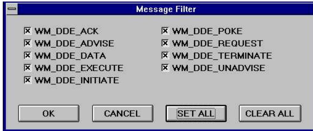
Figure 169. In the Set Message Filter dialog, select the messages on which you want DDE Spy to report.
