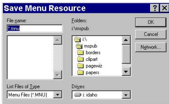
Figure 121. On the Save Menu dialog, specify the resource file to which you want to save the menu.
