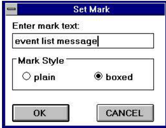
Figure 179. With the Set Mark dialog, you can annotate the event list by entering text and choosing a mark style.
