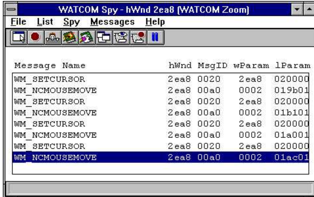
Figure 152. Once you start spying, the message list displays the messages selected for monitoring.
