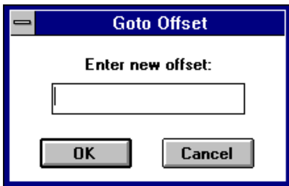
Figure 186. In the Goto Offset dialog, enter the offset you want to appear at the top of the Memory Display window.
