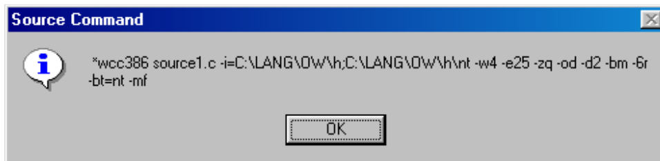
Figure 25. The IDE Source Command dialog displays the makefile commands for the selected source file(s).
