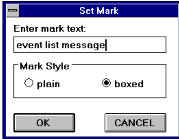
Figure 167. With the Set Mark dialog, you can annotate the event list by entering text and choosing a mark style.
