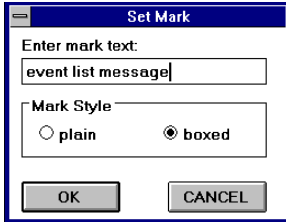
Figure 153. With the Set Mark dialog, you can annotate the message list by entering text and choosing a mark style.
