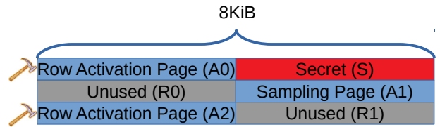
(b) Single-sided Rambled. Here, the sampling page (A1) is neighbored by the secret-containing page (S) on a single side.
