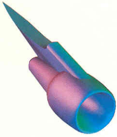
Jet engine modeled with two NURBS surfaces and rendered with four light sources.
