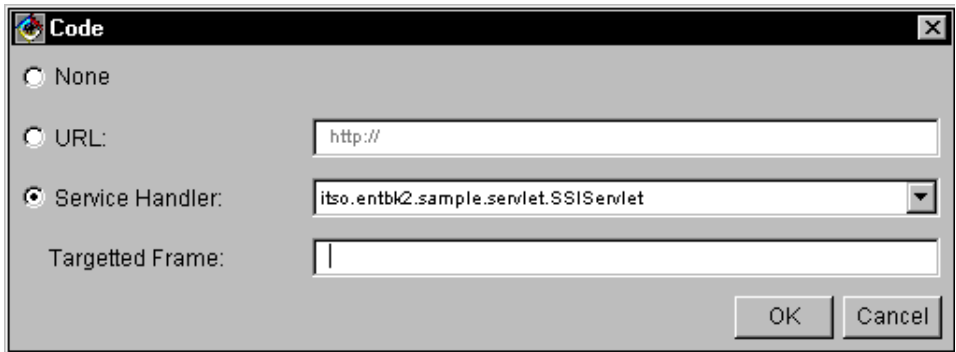
Figure 38. Code Property for a Server-Side Include Servlet
