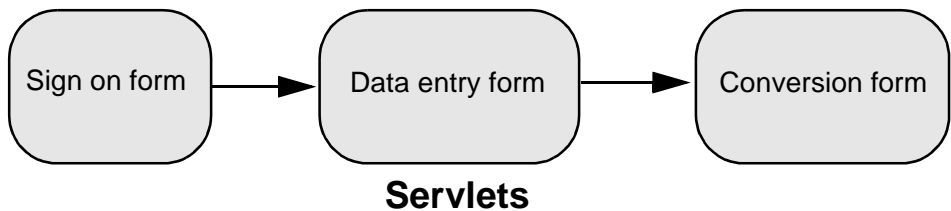
Figure 44. Servlet Chaining in Single Flow
