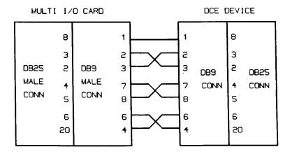
If the external serial device does not use Clear to Send (CTS) and Data Set Ready (DSR), wire the cable as follows:
