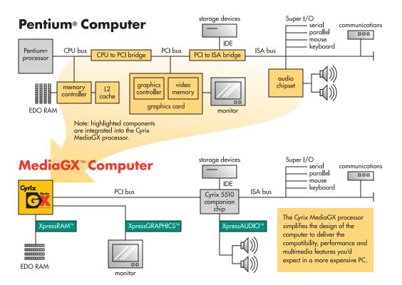
adding costly video memory. Just select the monitor resolution through Windows, and the MediaGX processor will automatically configure the rest.
