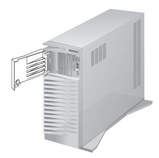
3. Remove the door by carefully lifting it up and off the hinges. Store it in a safe place.
