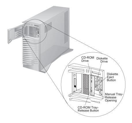
*Note:* If the CD-ROM tray does not extend out, insert the end of a paper clip into the manual tray-release opening and gently pull the tray open.
