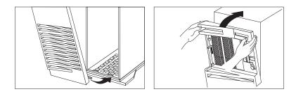
8. Reinstall the door at the front of the server by aligning the pins with the hinges, and sliding the door down.
