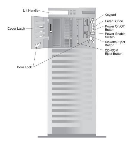
**Door Lock:** You can lock the door on your server to deter tampering with the internal components.
