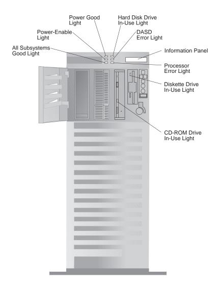
**All Subsystems Good Light:** This green light indicates that all subsystems are functioning properly.
