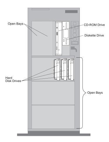
**Hard Disk Drives:** The number of preinstalled drives and their capacities vary by model.
