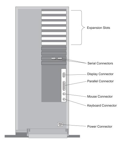
**Expansion Slots:** The PC Server 720 has seven expansion slots accessible from the rear of the server. A SCSI-2 adapter comes preinstalled in one of the expansion slots. The six remaining slots are available for expansion. You can add PCI or Micro Channel adapters to provide communication, specialized graphics, and sound. Many adapters provide bus-master capabilities, which enable the adapters to perform operations without interrupting the system microprocessor.
