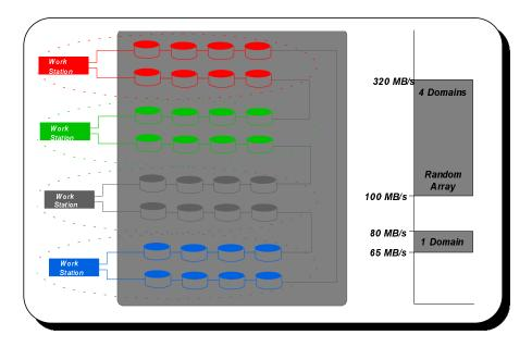
By contrast, FC-AL cannot scale performance due to the effects of arbitration. Only a single drive can be communicating with a single initiator on an FC-AL loop at one time. So, showing the same configuration in FC-AL would give you a maximum theoretical performance of 100 MB/s. This is depicted in the figure below.
