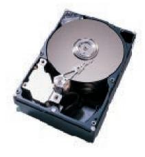
Ultrastar 18XP 3.5-inch 18.2 GB 7,200 RPM disk drive
